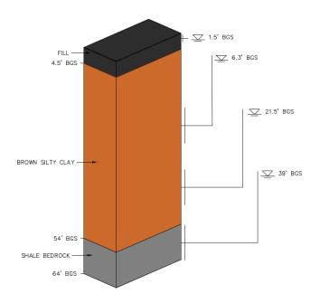
The schematic is to scale showing the relative thickness of clay between the fill and the underlying bedrock. The depths to water shown on the right side of the schematic are typical although at several locations across the BCP Site there is discontinuous saturation in the fill layer.
